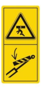
Stay clear of swinging range folding machine parts!
